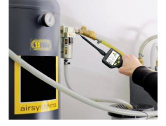
**Note**: The focus tube and tip are used to pinpoint the leak area. Do not use them in measuring flow leak.
