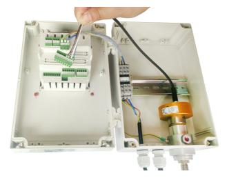
1. Open the S305 case and remove the sensor cable connected at the display terminal first. See the left picture.
