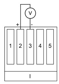
**C.** loop powered 4 ... 20 mA sensor with supply from S320
