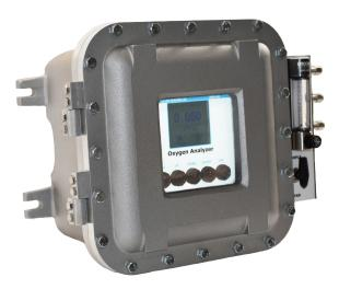
The OMD-690 is designed to measure trace oxygen in a Class 1, Division 1 groups B, C, D hazardous area. The unit combines an advanced set of electronic features with our industry leading precision electrochemical oxygen sensor technology in a fully explosion-proof ATEX certified enclosure. The result is a highly reliable and cost effective design with an easy-to-use user interface.
